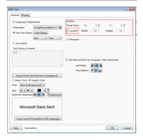
When the text includes a lot of words and characters, the revolving displaying function can be used to save the space. The revolving displaying function can be used by checking the "Marquee" function. The moving direction and the revolving displaying speed can be set in the properties dialog of the static text.
