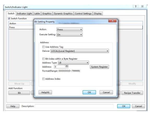
The default action is "Press". The default Execute Setting is "On". The default address is "LBO". They are modified into the required as follows.
