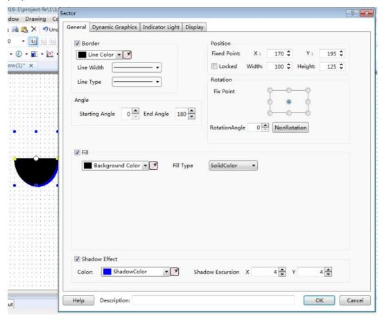
A sector can be got by setting the properties such as line color, width, type, starting angle, end angle, position, rotation, fill color, fill type and shadow effect. It can be freely drawn by dragging the yellow and blue areas.
