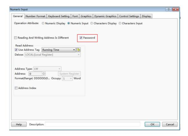
When the "Password" is checked, "\*" will be displayed in the component (See the figure below). It can be checked if the current component is used to input the password.
