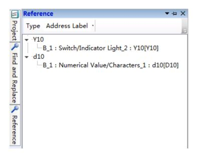
For example, all the uses of "Address" in the current project are listed in the following after selecting it.
