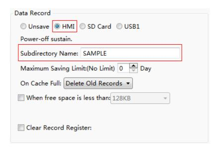
The "Maximum Saving Limit" option is set "0" Day by default. That means that there is no limit to save. However, there is a limit because of the limited capacity of the HMI Flash. It is suggested that the "Maximum Saving Limit" option is set several days when you select HMI to save data, such as 15 days, 30 days, and so on.
