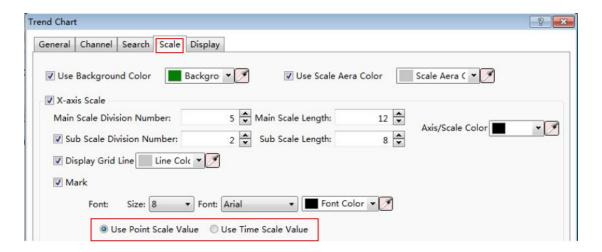
The option "Use Point Scale Value" means that the values of the sampling data points are used as the X-axis scale. The option "Use Time Scale Value" means that the time of the data sampling is used as the X-axis scale.
