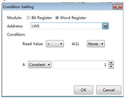
There are two pop-down lists in the Condition setting area. The first list is used to select the compare relationship. The compare relationship symbols include "<", ">", "<=" ">=", "==" and "! =". The second list is used to add the next condition of the word register LW0. The default of the second list is "None". It means that there is not the next condition any more. You can select "AND" or "OR" in the second list. It means the relationship between the current condition and the next condition.
