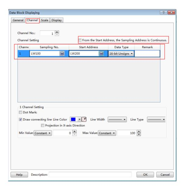
The below parameters setting for the selected channel is same to the Trend Curve or the XY Chart. Please refer to the settings in the "Channel" property TAB of the Trend Graph or XY Curve.
