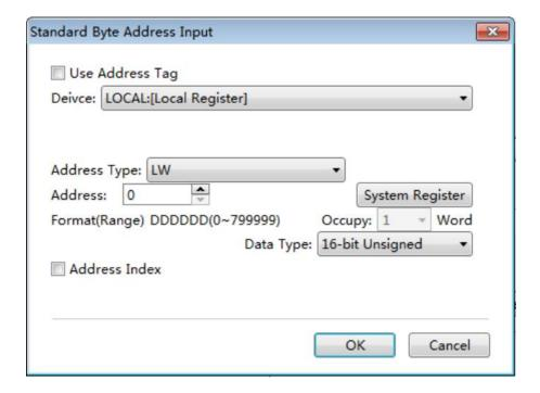
In the HTP Designer software, the corresponding byte or word addresssymbolsare given according to the various connected devices. For the PENTAX FL2N series PLC,D represents the data register,SD represents the special address, represents the timer, C\_word represents the 16-bits counter which saves the current value, and C\_dword represents the 32-bits counter which saves the current value. As shown as below.
