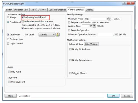
After checking the option "Indicating Invalid Mark", the prohibited mark will display on the component if the operating conditions are not met. The prohibited mark is shown as below.
