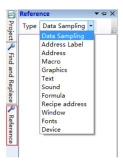
For example, all the uses of "Data Sampling" in the current project are listed in the following after select it.
