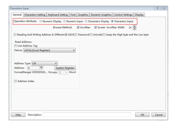
The "Operation Attribute" includes four operation types: "Numeric Display"," Numeric Input"," Character Display" and "Character Input". If you want the current Character Input component change to the Character Display component or Numeric component, you can modify it here. It is highly efficient for the project modifying and maintaining.
