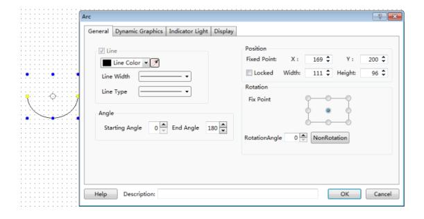
An arc can be got by setting the properties such as line color, width, type, starting angle, end angle, position and rotation. It can be freely drawn by dragging the yellow and blue areas.
