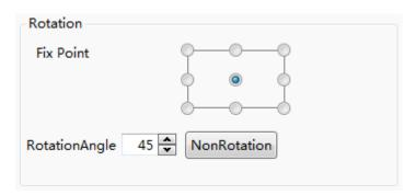
The function of "Rotation" can adjust the display angle of the components such as static graphics, vector graphics and other components. This function is a static function. That is, the display angle is not adjusted in the HMI if you set the display angle in the "Rotation" property. If you want to dynamically adjust the display angle of the graphics, please refer to: Detailed manual/General functions/Dynamic Graphics.
