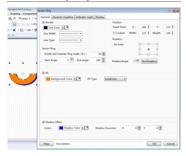
A sector ring can be got by setting the properties such as line color, line width, line type, starting angle, end angle, position, rotation, fill color, fill type and shadow effect. It can be freely drawn by dragging the yellow and blue areas.
