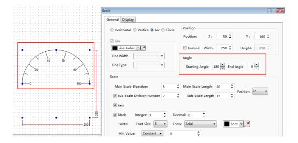
For the option "Position" in the "Scale" property box, the axis position of the sacle can set "In", "Out" and "Center".
