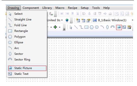
After the static picture component is selected, drag by the left key of the mouse, and then the corresponding properties window will pop up.
