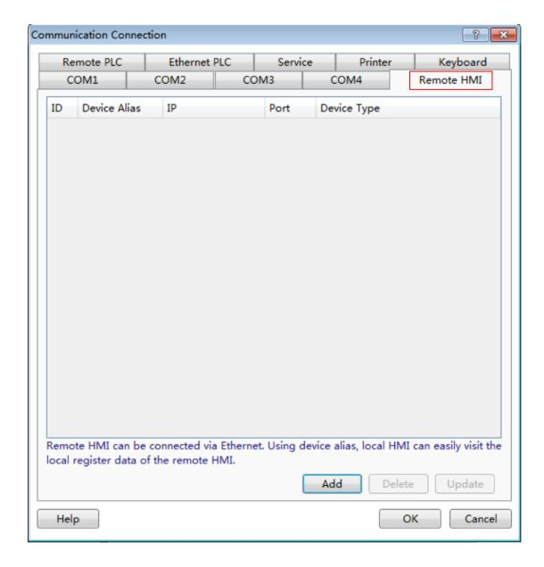
For one of the HMI device, anyone of other HMI devices in the same Ethernet network of the LAN is the Remote HMI. For example, there are two HMI: one named HMI1, another one named HMI2. These two HMI devices are connected in an Ethernet network. For HMI1 device, HMI2 is the "remote HMI" of HMI2. For HMI2 device, HMI is the "remote HMI" of HMI2.
