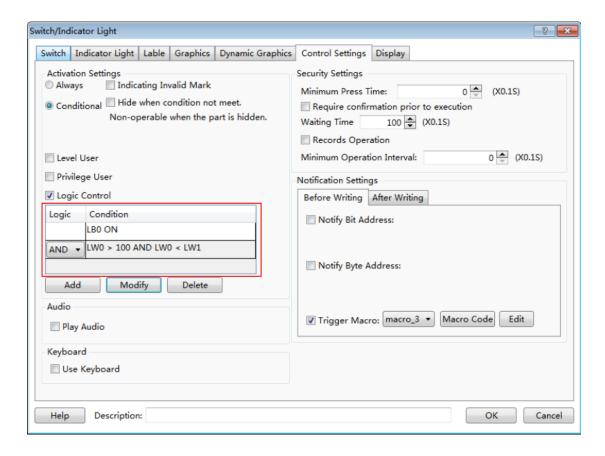
There is a relationship option in front of the second condition in the Logic Control list. The option can be set "AND" or "OR". It means the logic relationship between the previous condition and the following condition. The component can be operated or display only if the result of all the conditions logic operation is true.
