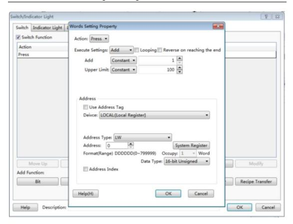
The type of "Execute Settings" includes "Add", "Subtract", "Increase", "Decrease", "Set Up Constants", "Set Up Character Strings", "Set Up Figures By Bit" and "Logic Operation".
