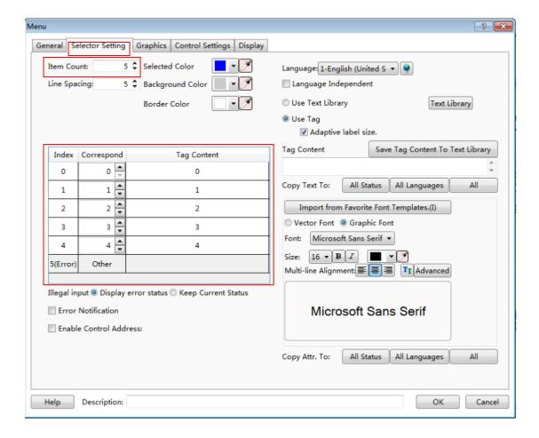
For example, the "Item Count" is set 5. The value of the "Index" is 0~5. Index 0~4 are corresponding to effective items and item 5 is corresponding to the "Error" one.
