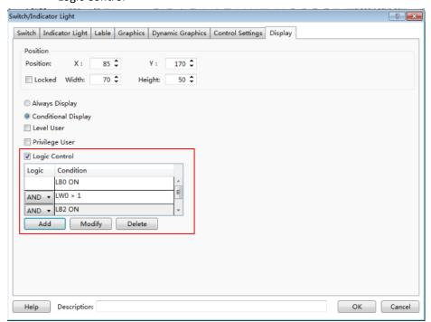
If you check this function, the component can be controlled to display according to the logic condition. The condition can be multiple logical operations.
