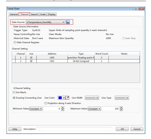
After you selecting a sampling data for the option "Data Source", all channels of this sampling data defined in the "Data Sampling" will be displayed in the "Channel Setting" property box.
