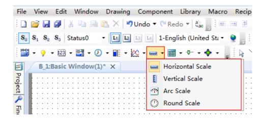
The "Horizontal Scale" is mainly used to display a progress bar. The "Vertical Scale" can be used to display the current liquid level of a tank or the charge state of a battery. The "Arc Scale" can display the value of a fuel meter, a speed meter, and other display devices. The "Round Scale" can display the revolution speed, the angle and other parameters.
