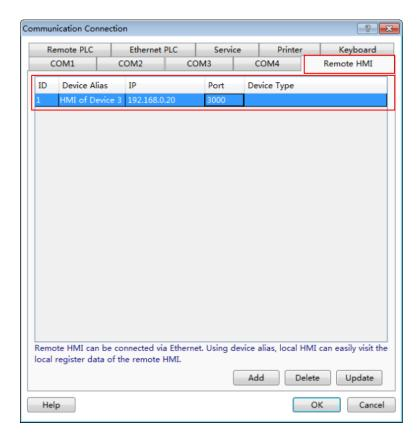
Click the button "OK" in the "Remote HMI" settings page to save, and then you can find the remote HMI device in the Device list of the register address. For example, it is shown as below.
