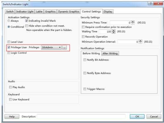
After checking this function, you need to login by using the corresponding user privilege to operate the component. It is shown as below.
