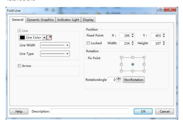
Click the left key to fix the fold line point in drawing. And click the right key to finish drawing. See details in: <a href="Detailed Manual/Drawing/Straight Line">Detailed Manual/Drawing/Straight Line</a>.
