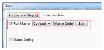
In this example, execute the "Computing" macro when the input value changes by using the timer function. See settings as shown as below. The detailed using method of the timer component, please refer to: <a href="Detailed manual/Component/Timer and Data">Detailed manual/Component/Timer and Data</a>
