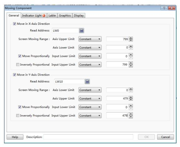
The option "Move in X-Axis Direction" refers to moving along the horizontal direction. The option "Move in Y-Axis Direction" refers to moving along the vertical direction. These two options can be checked together. That means moving in an oblique line direction. The angle of the oblique line can be computed based on the moving distance along the x-axis and along the y-axis.
