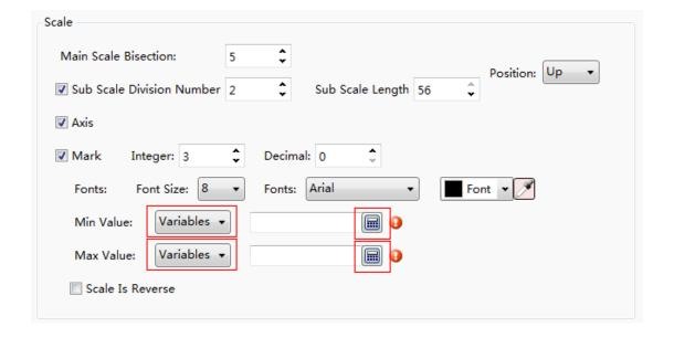
Usually, the scale value is displayed increasing from left to right. Sometimes, it needs to be displayed increasing from right to left. To do that, you should check the option "Scale Is Reverse".
