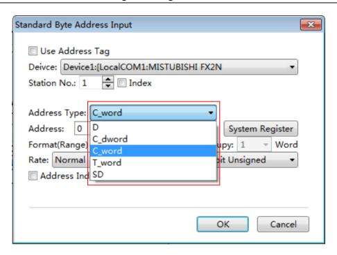
If the address is not connected with the device after you inputting a specific address number, you should check whether the parameters (such as Device, Station No. and Address) are set correctly. For example, these parameters are set as follows.
