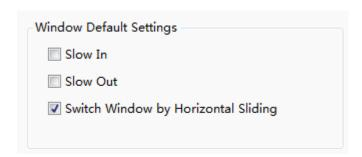
After the "Switch Window by Horizontal Sliding" option is checked, the windows can be switched by horizontal sliding action. This function is only supported by the capacitive HMI devices.
