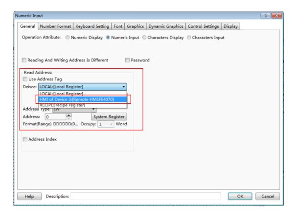
After finishing setting the "Remote HMI", the local HMI can access all the registers of the "Remote HMI", including the LW, RW, SRW, LB, SRB and other registers.
