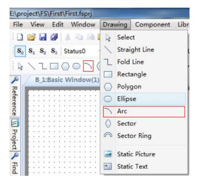
Select the arc component, designate any area to draw, and double click to set the arc properties.
