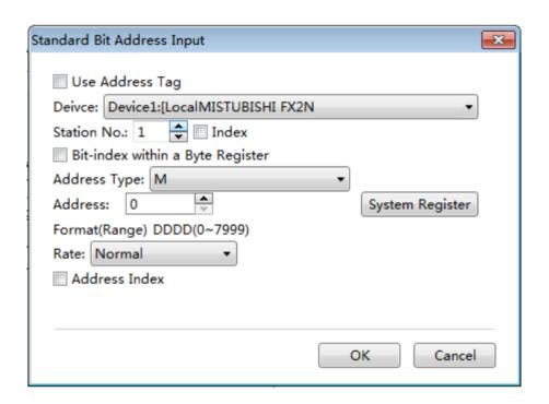
In the HTP Designer software, the corresponding bit address symbols are given according to the various connected devices. For the MITSUBISHI FX2N series PLC, X represents the input address, Y represents the output address, M represents the middle register address, SM represents the system special bit address, and S represents the state address. As shown as below.
