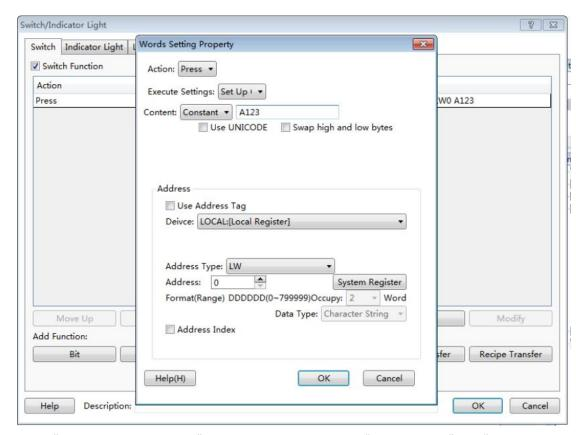
"Set Up Character Strings" has two optional attributes "Use UNICODE" and "Swap high and low bytes". When "Use UNICODE" is checked, it means the character string written to registers is coded by UNICODE. The string is normally displayed only in "UNICODE". If "Swap high and low bytes" is checked, the high and low bytes in the character string will be exchanged before written to the word register.
