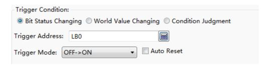
The "Trigger Condition" supports "Bit Status Changing", "Word Value Changing" and "Condition Judgment". The settings are referred to: <a href="Detailed manual/Component/Timer">Detailed manual/Component/Timer</a> and Data Transmission/Timer.
