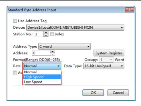
Certainly, you can use the address tag library. You need to prepare the data addresses in the address tag library before using them. Check the "Use Address Tag" in the "Standard Byte Address Tag" window and click the button "Open the "Address Tag Library" window. Select the byte or word address you need in the address tag library, as shown as follows.
