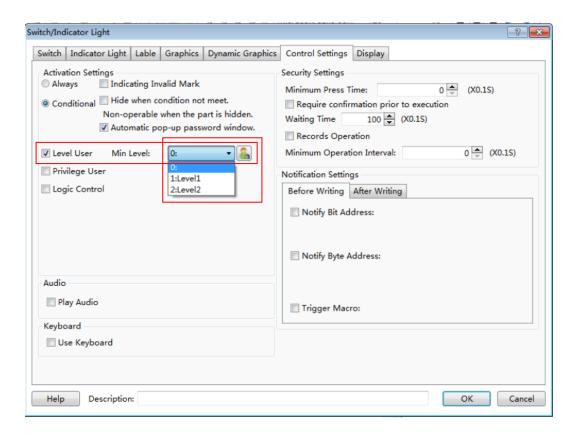
Run the project.A "User level login" window will pop up when you click the component. It is shown as below. You can operate the component only by entering the correct password in the "User level login" window.
