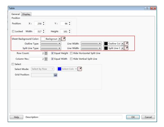
The option "Row Count" and the option "Column No." are used to set the number of the rows and the columns of the table. The option "Equal Height" and the option "Equal Width" can be checked. If they are all checked, the table will be a fixed-width table.
