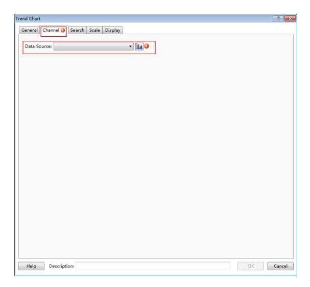
In the "Channel" property TAB, you need select a sampling data as the "Data Source". There will be a red exclamation mark here if the "Data Sampling" is not set. You can open the "Data Sampling" settings page to set the required sampling data by click the button
