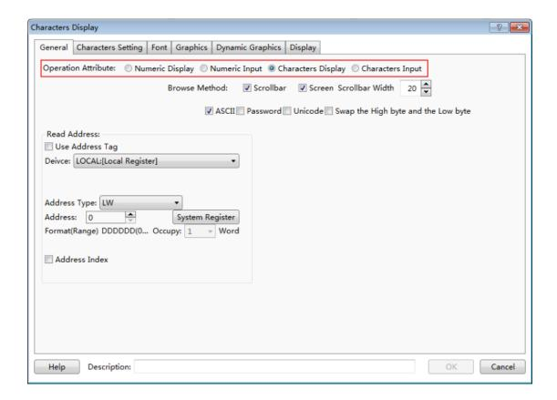
The "Operation Attribute" includes four operation types: "Numeric Display"," Numeric Input", "Character Display" and "Character Input". If you want the current Character Display component change to the Character Input component or Numeric component, you can modify it here. It is highly efficient for the project modifying and maintaining.
