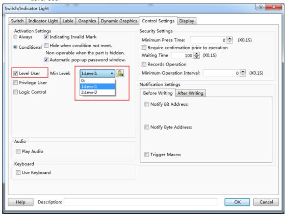
After checking this function, you need to enter the appropriate user level password to operate the device. It is shown as below.
