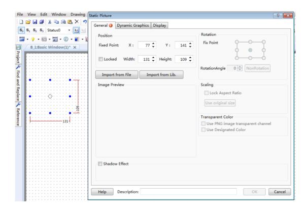
Local picture in the computer or in the software picture library can be imported by clicking the "Import from File" button or the "Import from Lib" button. And the picture will be put into the window by clicking the "OK" button.
