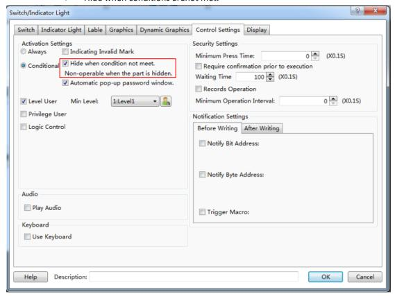
When you check the option "Hide when conditions are not met", the component will hide if the operating conditions are not met.
