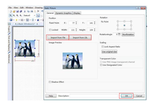
The static picture position can be modified. You can change the position by manually dragging or by setting the coordinates in the static picture properties window. The static picture size can be modified, too.
