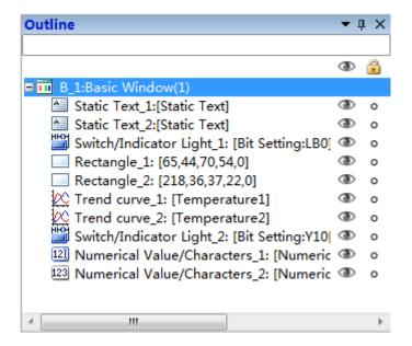
The tool button " on the top right corner which is used to control the display mode of the outline window. The tool button " is used to make the outline window show or auto hide. The tool button " x " is used to close the outline window.
