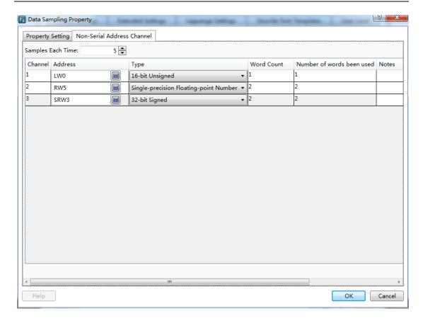
It can be seen that the sampling addresses of multiple channels could be non-continuous addresses.
