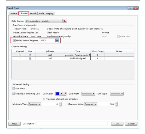
For example, the option "Hide Channel Register" is set LW500. Then the curve of Channel 1 is hidden when the bit 0 of the LW500 is ON. The curve of Channel 2 is hidden when the bit1 of the LW500 is ON.
