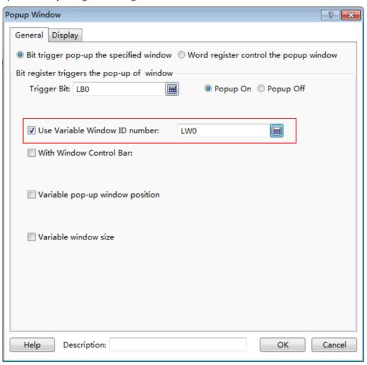
For the above example, the word register is specified LW0 and a numeric value input component is connected with LW0. The simulation running result is shown as below. Enter the corresponding window ID number in the numeric value input component and then click the button "Popup the window", the designated window will pop up.
