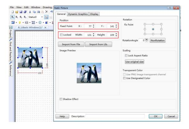
The static picture size and position can be fixed if the "Locked" is checked. And the static picture can be rotated around a fixed point. The fixed point and rotation angle can be set. The picture can be manually rotated (in any angle) after the fixing angle is set.
