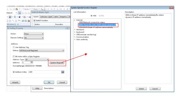
Certainly,the screen is connected with multiple slaves at sometime. The station number is varied. At this moment, you need to use the Index function. This function uses a word address to provide a variable station number. The setting process is shown as follows.
