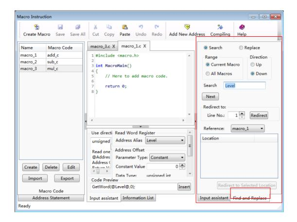
Find and Replace function can provide a more convenient method of editing the macro codes. It can perform jump between lines and you can view the macro reference here.
