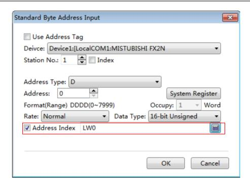
In addition, there are many system special function register addresses. You can quickly select one by clicking the button "System Register", as shown as follows.
