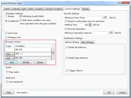
After check this function, the component can be operated when the specified conditions are satisfied. The conditions can be multiple logical operations.
