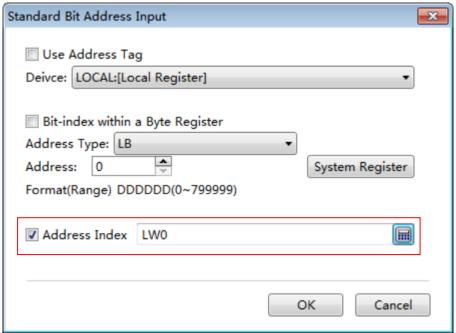
In addition, you can use the System Register in the Standard Bit Address Input window. When you click the System Register button, the System Special Function Register window will pop up. There are many system special function register addresses in this window, as shown as follows. You can quickly select one to use.
