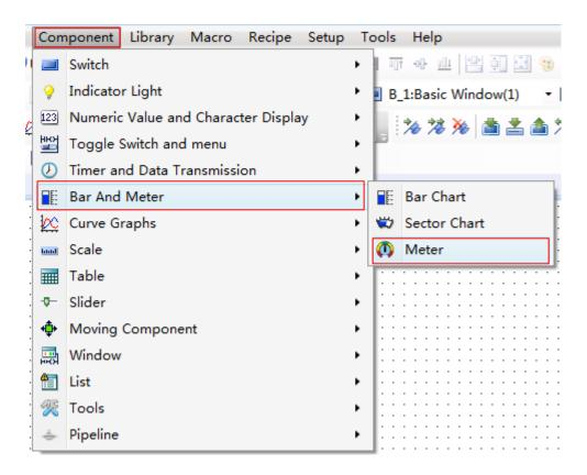
You can add a Meter component by clicking the corresponding tool button in the shortcut tool bar. It is shown as below.
