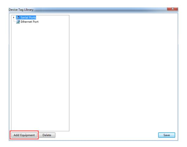
**Add Equipment**: Click the "Add Equipment" button, select the "Serial Port Type", and select the "Manufacturer" and "Device Type". Then click "OK" to finish adding after selecting device, the added device should be the tag type device here, such as the figure shown as below.
