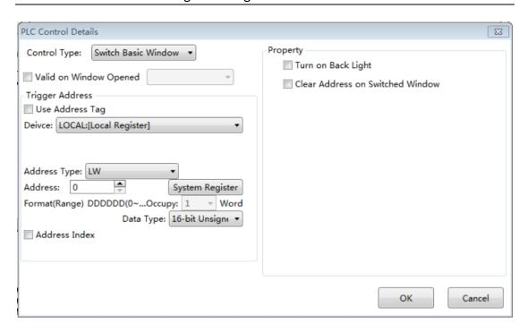
The "Control Type"refers to the action of the "PLC Control". It includes "Switch Basic Window", "Report Current Window No.", "Back Light Control", "Execute Macro Instruction", "Audio Control", "Sheet Print", and "Force Buzzer off".
