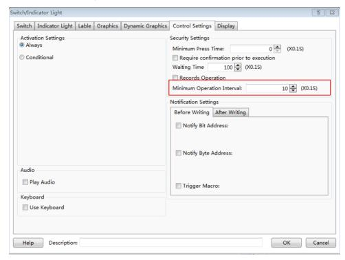
By using the "Minimum Operating Interval" function, continuous actions can be avoided in a short time due to touching the screen continuously by mistake.
