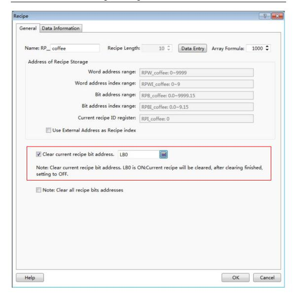
For example, if the value of the "RPI\_ coffee: 0" register is 3, the data of the No. 3 group of the recipe "RP\_coffee" will be cleared when the "Clear current recipe bit address" LB0 is set ON. After finish clearing,LB0 will be reset OFF.
