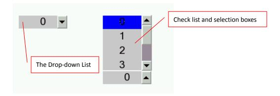
The figure above shows that when the "The Drop-down List" completes operation or has no operation, it is "withdrawn". It will be unfolded only when it is operated, while the "Check list and selection boxes" is always unfolded no matter it is in operation or not, and it can be directly viewed and operated.
