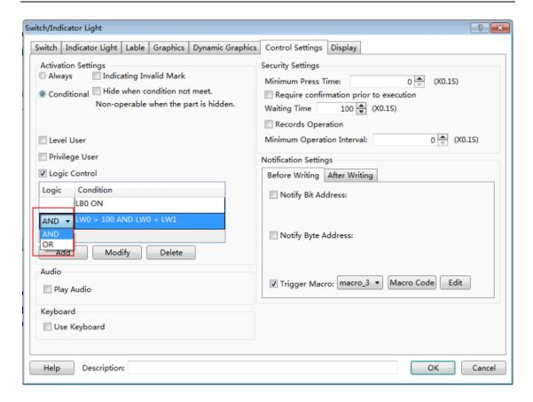
There are the button "Modify" and the button "Delete" besides the button "Add" in the Logic Control list. After selecting a condition in the Logic Control list, you can click the button "Modify" to edit it again or click the button "Delete" to remove it from the Logic Control list. You can also double-click a condition in the Logic Control list to modify it.
