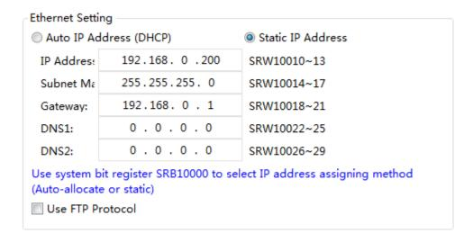
When SRB10000=0, the setting mode is DHCP. When SRB10000=1, the "Static Address" mode is used to assign the IP address. You can switch the IP address setting mode by the SRB10000 register.
