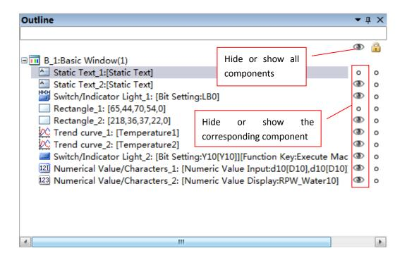
When you click the right tool " ", it will change to " and lock the corresponding component in the window. When you click it again, it will change to " " and unlock the corresponding component. The top tool " " will control all components locked or unlocked by clicking it. The component will not move if it is locked.
