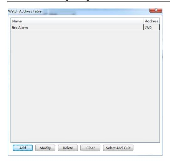
**Add**: You can add new watch address entry. Click "Add", set the watch address name, such as "Fire Alarm", and set the address of the watch entry, such as "local register LW0",set the data format, there are various data types to choose; click "Confirm" after setting finished, you can see the figure as below.
