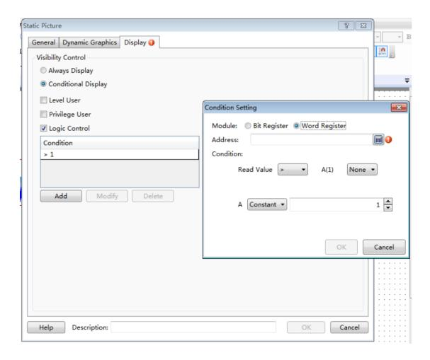
The static picture can be converted into a dynamic one by logic control. Static pictures can be quickly switched by picture stacking and the control address.
