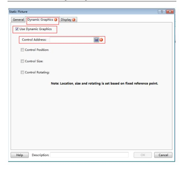
When the control address is fixed, the position, size and rotation can be controlled. E.g.: when there are many sector pictures, they can be set to display rotating effect by setting the Control Rotating.
