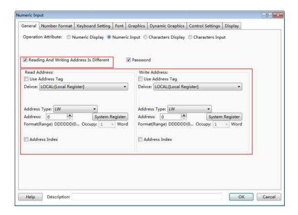
The numeric value input component is integrated with functions of reading data from an address and writing data to an address. When the "Reading And Writing Address Is Different" is not checked, the using method is same to the "Numeric Value Display" component. When the "Reading And Writing Address Is Different" is checked, different address can be set in the "Read Address" and in the "Write Address".
