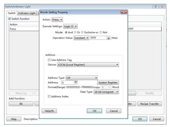
In the figure above, when the component is operated, the value in register LWO will has a logic operation "And" with 0×FFFF. The logic result will be written to register LWO. The operations of otherthree modes are similar to "And" mode but the logic operation.
