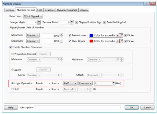
The data can be logically operated by the component which the logic operation can be "And", "Or" or "Exclusive or". And the result of logic operation will be displayed.
