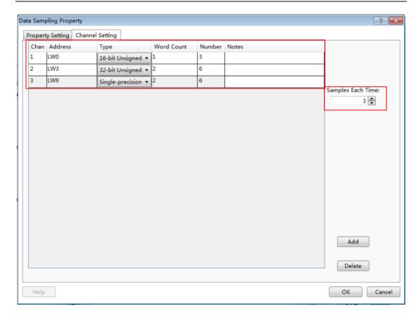
In this example, LW0  $\sim$  LW2 is occupied by the first channel, LW3  $\sim$  LW8 is occupied by the second channel, and LW9  $\sim$  LW14 is occupied by the third channel. The number of addresses is three times as the number which the "Samples Each Time" is set 1.
