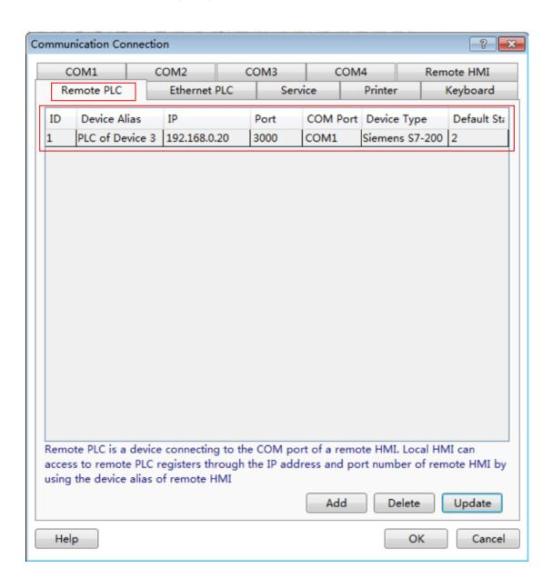
You can find the remote PLC device in the "Device Type" of the component. For example, it is shown as below.
