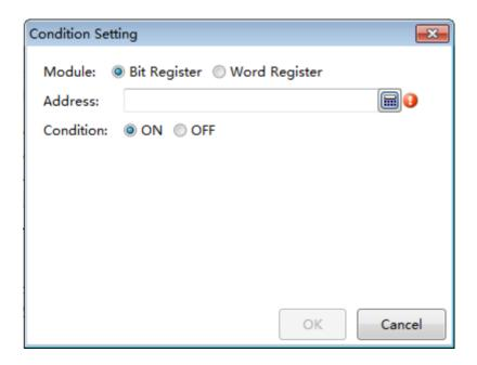
There are two address types: Bit Register and Word Register. The default selection is Bit Register. The logic condition judgment for Bit Register is "ON" or "OFF". The default selection is "ON". Click the tool button " or double-click the "Address" blank box,
