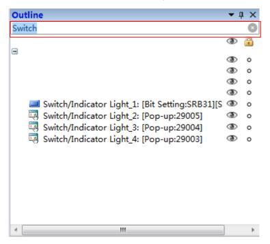
When you click the little eye tool " " except the top one, it will change to " " and hide the corresponding component in the window. When you click it again, it will change to " " and make the corresponding component show in the window. The top little eye tool " " will control
