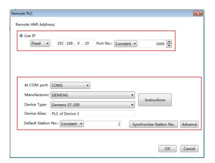
Click the button "OK" to confirm the settings and the "Remote PLC" device is added to the "Remote PLC" settings page.
