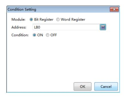
The red exclamation mark will disappear after you select an address for the condition. Click the button "OK" and the condition will be added to the Logic Control list. It is shown as below. It means the current component will be valid when the bit register LB0 is ON.
