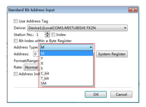
If the address is not connected with the device after you input a specific address number, you should check whether the parameters (such as Device, Station No. and Address) are set correctly. For example, these parameters are set as follows.
