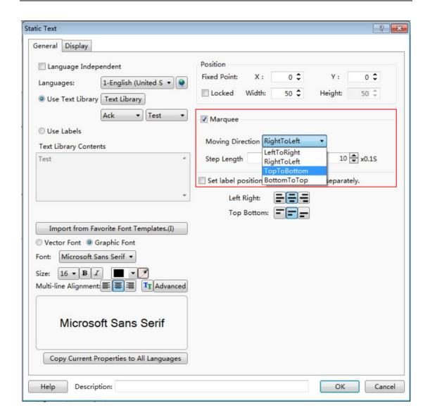
Similar to static picture functions, the static text can be also set to display only if necessary. The user can choose that the static text is displayed all the time or displayed in conditions by setting the Display properties. The conditional display type includes Level User, Privilege User and Logic Control.
