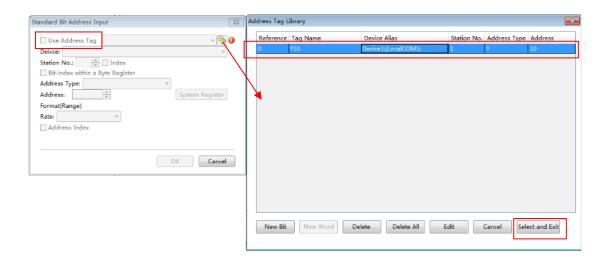
The "Bit-index within a Byte Register" function can be used. You need to check the "Bit-index within a Byte Register", as shown as below.
